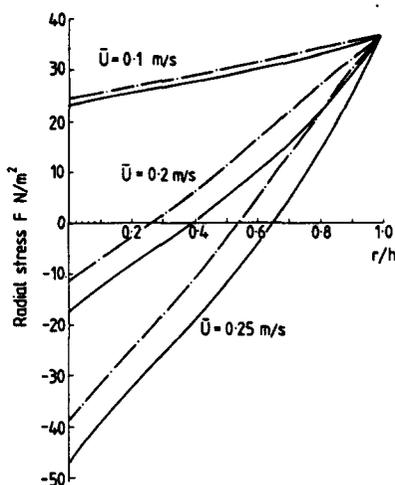
Figure 7. Effect of film velocity profile on radial stress distribution. Water temperature = 20°C; film thickness = 1 mm; corner radius = 1 mm; —, linear velocity profile (shear-driven film) - - -, parabolic velocity profile (gravity-driven film).
