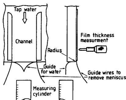
Figure 9. Apparatus for gravity driven film flowing around a corner.
