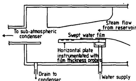
Figure 10. Low pressure steam tunnel for horizontal film flow around a corner.
