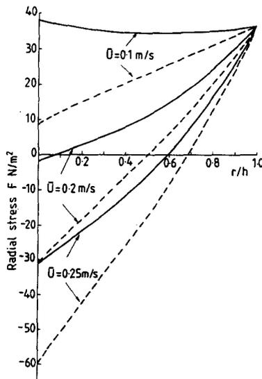
Figure 3. Effect of film velocity on radial stress distribution. Water temperature = 20°C; film thickness = 1 mm; Corner radius = 1 mm; ———, gravity assisting film attachment; - - - - -, gravity opposing film attachment.
