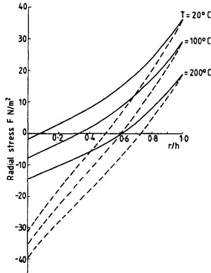
Figure 6. Effect of film temperature on radial stress distribution. Mean film velocity = 0.2 m/s; film thickness = 1 mm; corner radius = 1 mm; ———, gravity assisting film attachment; - - - - - , gravity opposing film attachment.
