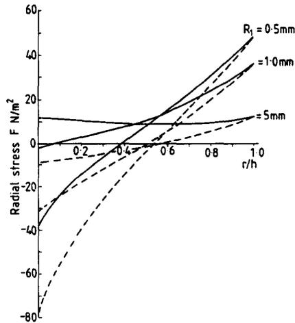
Figure 4. Effect of corner radius on radial stress distribution. Water temperature = 20°C; mean film velocity = 0.2 m/s; film thickness = 1 mm; ———, gravity assisting film attachment; - - - - - , gravity opposing film attachment.
