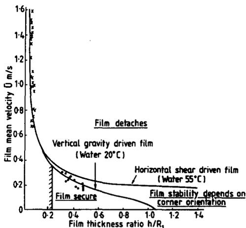
Figure 8. Critical film flow around 1.5 mm radius corner. —, theoretical curve; X, experimental data for horizontal shear-driven film; ●, experimental data for vertical gravity-driven film; † minimum film thickness of gravity driven film (Mikielewicz and Moszynski 1976).
