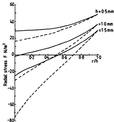
Figure 5. Effect of film thickness on radial stress distribution. Water temperature = 20°C; mean film velocity = 0.2 m/s; corner radius = 1 mm; ———, gravity assisting film attachment; - - - - - , gravity opposing film attachment.
